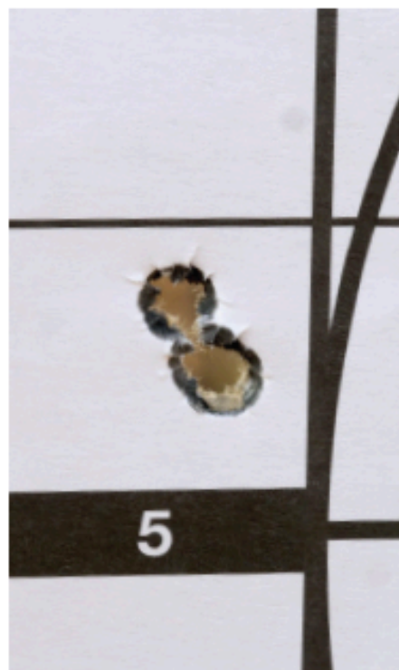
The provided AllTerra handloads with Hornady 143-grain ELD-X bullet resulted in a three-shot group that went 0.252-inch.
