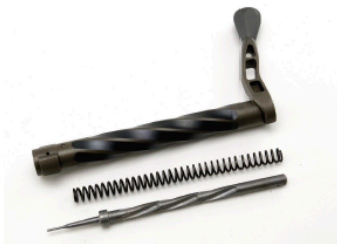
Within the bolt body stands an oversized firing pin body that is also fluted. Why? To reduce weight and lock time.
