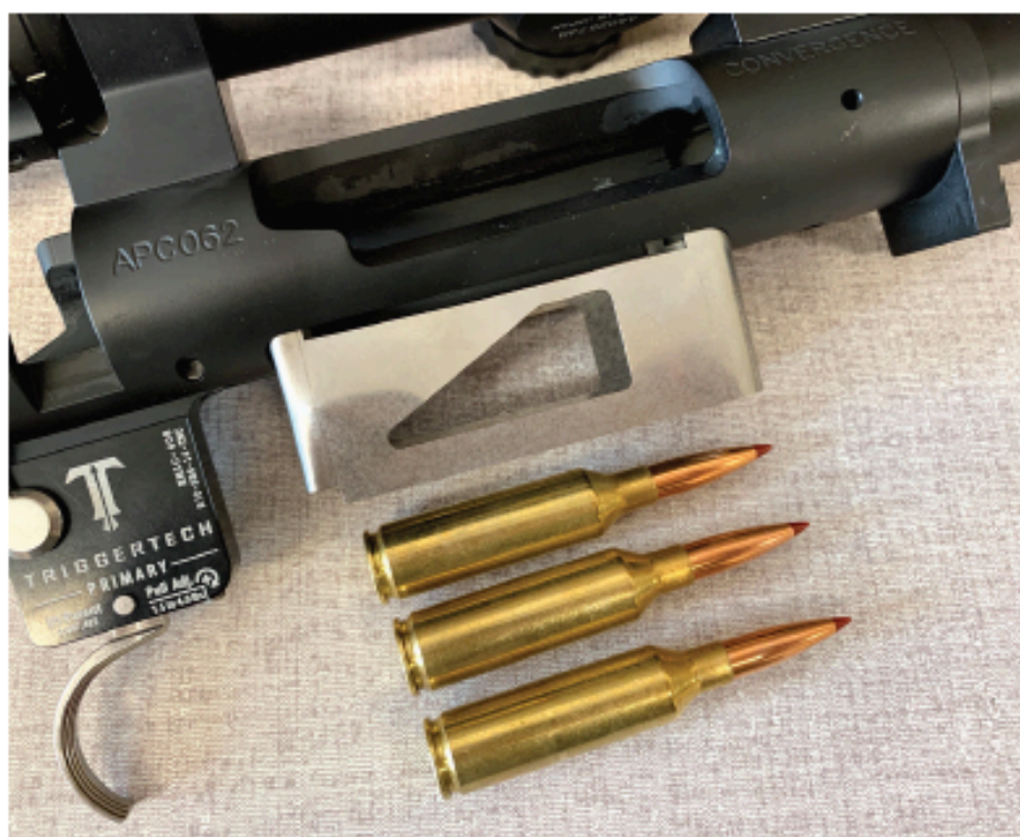
A one-piece, aluminum, hinged floorplate secures a 3-inch-long metal box magazine that holds three 6.5 PRC cartridges ready for action.
