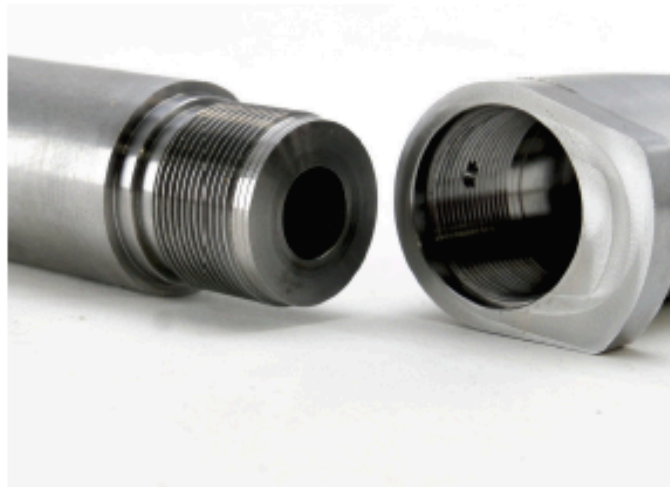
The front receiver ring is specially cut with two mortises into which the specially turned barrel tenons mate perfectly via 20-pitch threads.
