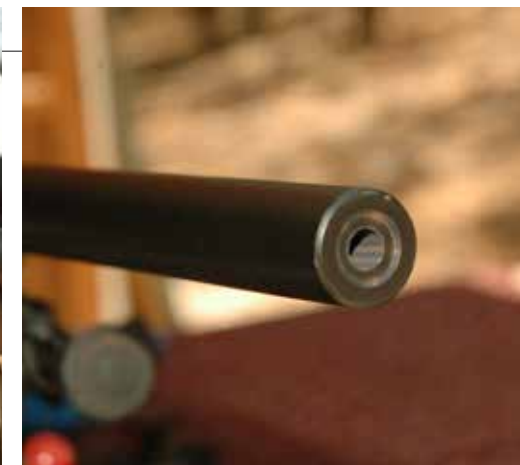
The muzzle crown is the last thing the bullet touches, and is often the culprit in accuracy problems. Diagnosing a sloppy or damaged crown is easy, and re-cutting a crown is a simple job.
