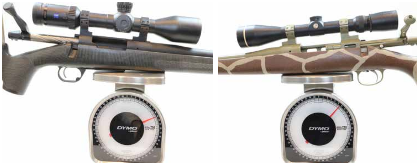
With full-size scope, stock, and a longer and/or stiffer barrel, it's difficult to make a really light mountain rifle. These two rifles probably define sensible weight range: The AllTerra (left), large scope and 25-inch medium-weight barrel weighs nine pounds; the MGA .270 (right), with slim 22-inch barrel, slender stock, and one-inch-tube scope weighs 5.7 pounds. Big difference, but it depends on what you like.
