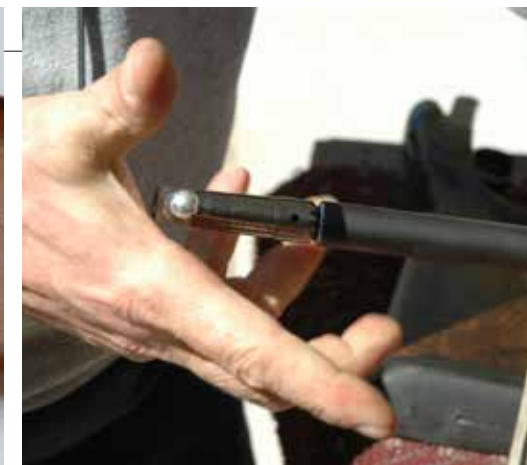
The muzzle crown is the last thing the bullet touches, and is often the culprit in accuracy problems. Diagnosing a sloppy or damaged crown is easy, and re-cutting a crown is a simple job.
