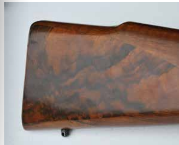
John Batten's .30-.338, made by R.A. Wells in about 1960, is stocked in large-slice laminate, almost unheard of back then. Laminated wood is probably the strongest of all gunstock material, but also heavier than solid wood or synthetic.
